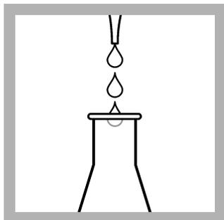
6. If the sample volume is 100 mL, add 2 mL of 8 N Potassium Hydroxide Standard Solution. If the sample volume is 50 mL or less, add 1 mL of 8 N Potassium Hydroxide Standard Solution.
