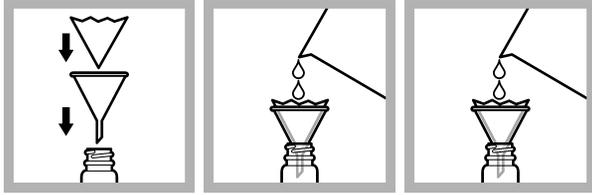
**1.** Put the filter paper in the funnel. Put the funnel on a bottle.
