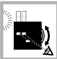
12. Hold the color comparator box in front of a light source. Turn the color disc to find the color match.
