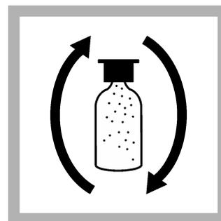
4. Quickly invert the AccuVac Ampuls several times to mix.
