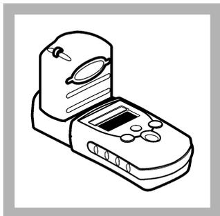
**13.** Install the instrument cap over the cell holder.
