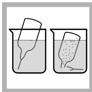
3. **Prepare the sample:** Pour at least 40 mL of sample in a 50-mL beaker. Fill the second SPADNS or SPADNS2 Fluoride Reagent AccuVac Ampul with sample. Keep the tip immersed while the Ampul fills completely.
