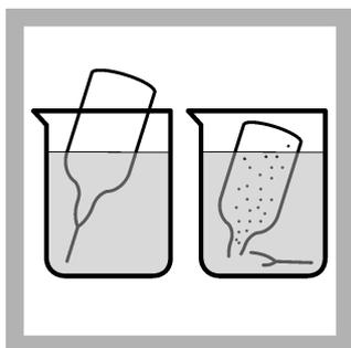
2. **Prepare the blank:** Pour at least 40 mL of deionized water in a 50-mL beaker. Fill one SPADNS or SPADNS2 Fluoride Reagent AccuVac Ampul with deionized water. Keep the tip immersed while the Ampul fills completely.
