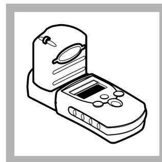
8. Install the instrument cap over the cell holder.
